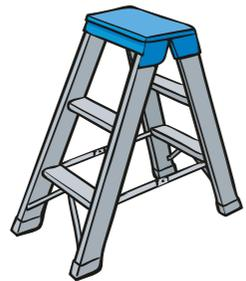
Step ladders should be fully opened and stay bars locked in place
